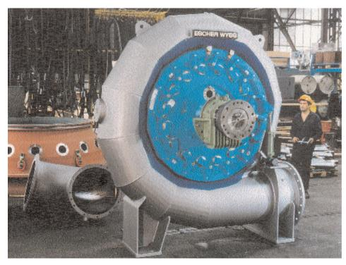
Horizontal spirally shaped Francis turbine for water power-station with RENK slide bearing EMZLA 18-180
