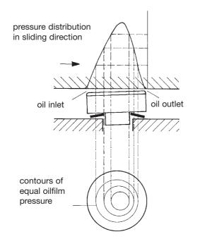
Figure 22 Pressure build-up at a tilting pad
