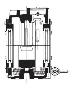
Figure 7 Slide bearing type SN
