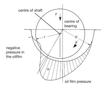
Figure 18 Pressure build-up in a plain cylindrical bearing
