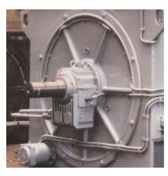
Asynchronous motor equipped with RENK slide bearing EFWLB 11-110
