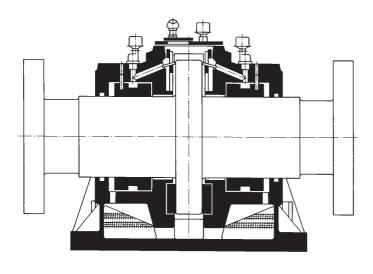
Figure 8 Slide bearing type DN
