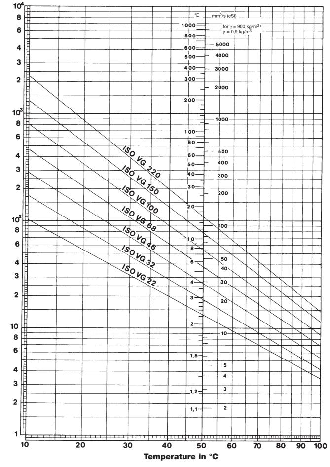
Figure 30 Viscosity-temperature-graph for mineral oils (with reference to G. Niemann and DIN 51 519)
