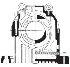
Figure 35 Bearing with water cooling
