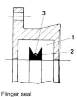
Figure 49 Flinger seal protection IP 22
