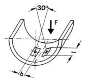
Figure 24-2 Execution with two lubricating pockets
