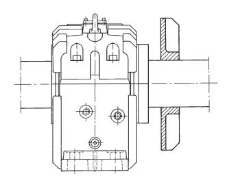
Figure 39 Arrangement of a cooling disc
