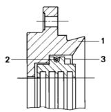
Floating labyrinth seal, type 10 protection IP 44
