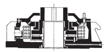
Figure 11 Slide bearing type VD
