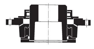
Figure 15 Slide bearing type EVF
