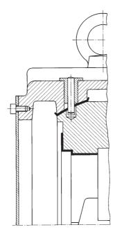
Figure 54 Insulation of the spherical seating
