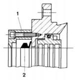
Floating labyrinth seal combined with bolt-on baffle, type 12, protection IP 55
