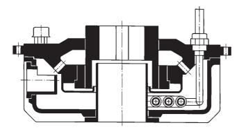
Figure 12 Slide bearing type VF
