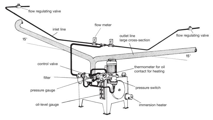
Figure 38 Diagramm of an oil supply system
