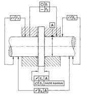
C Shaft with solid collar for journal/ thrust bearing loads in both directions
