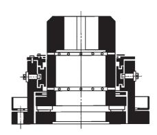
Figure 14 Slide bearing type EVE
